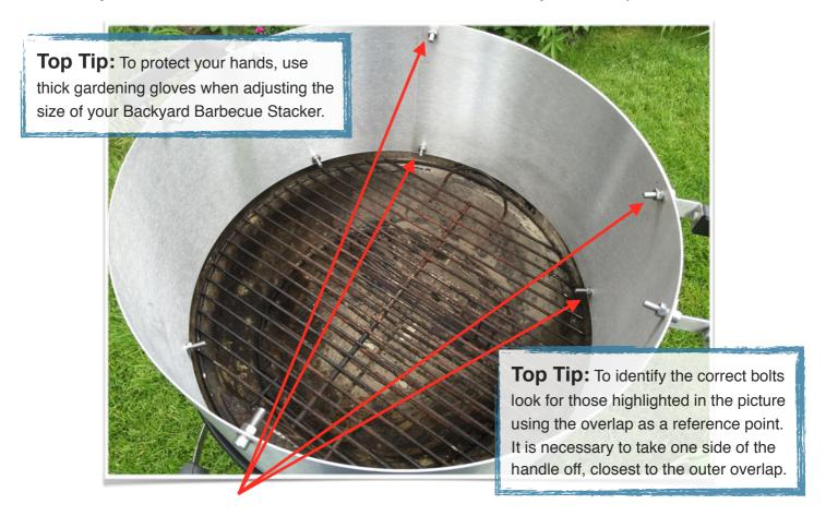
1) Undo the bolts highlighted using a 10mm spanner (wrench) and 5mm Allen key, keep them close as they will be needed again. The Backyard Barbecue Stacker is supplied with an extra set of bolt, washers and nut. These will be required when making the Backyard Barbecue Stacker fit a 57cm barbecue.
